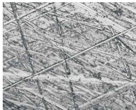
Sample after grinding with Platinum I disc.
