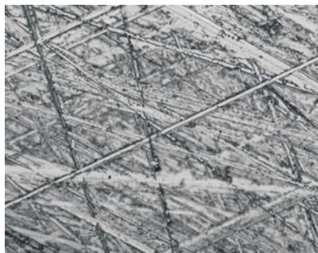
Sample after grinding with Platinum I disc.
